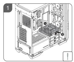
\*(Fan and fan mount needs to be removed completely)
